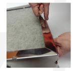
Grab one handle and the back of the frame and pull to separate the components.
